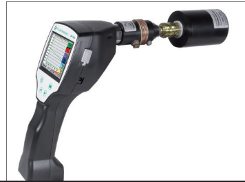
Dry container - for sensor protection and quick adaption time
