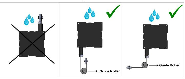
4. The wire should not be pulled in angular. If needed, please use guide rollers.
